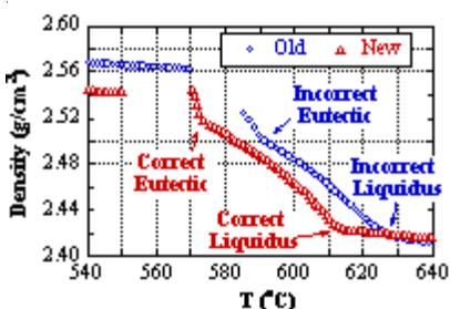
Comparison of dilatometer results obtained with the new and old setup
